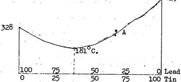
It is apparent that the 63 - 37% mixture has a very much lower melting point at 181 deg.C. than Lead at 328 deg. or Tin at 419 Deg.C. This point is known as THE EUCTECTIC POINT.
